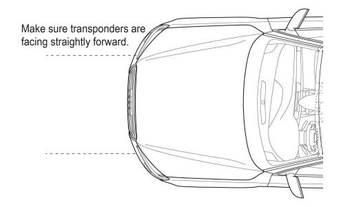
Make sure transponders are horizonally installed by level included in the package.
